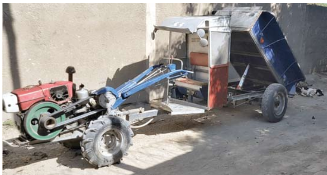
A two-wheel tractor with an improved driver seat and hydraulic tipping trailer system in Beyene Chufamo's workshop in Meki, Ethiopia. (Photo: CIMMYT)
